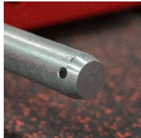
Tapered Pin for easy adjustment
